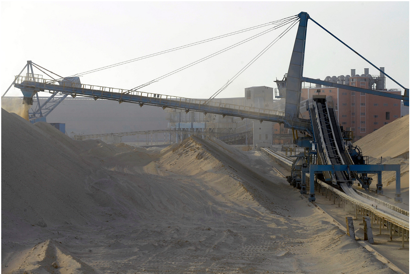
Photo above: Untreated phosphate being dropped off at the end of a conveyor belt at the OCP's Marca factory, near Laayoune, Western Sahara, on May 13, 2013. Photo by FADEL SENNA/AFP via Getty Images.
